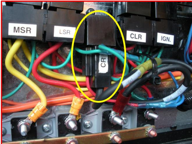
**Step 12**: Use a tie wrap to secure relays into receptacles. Being careful not to disturb electrical connections.
