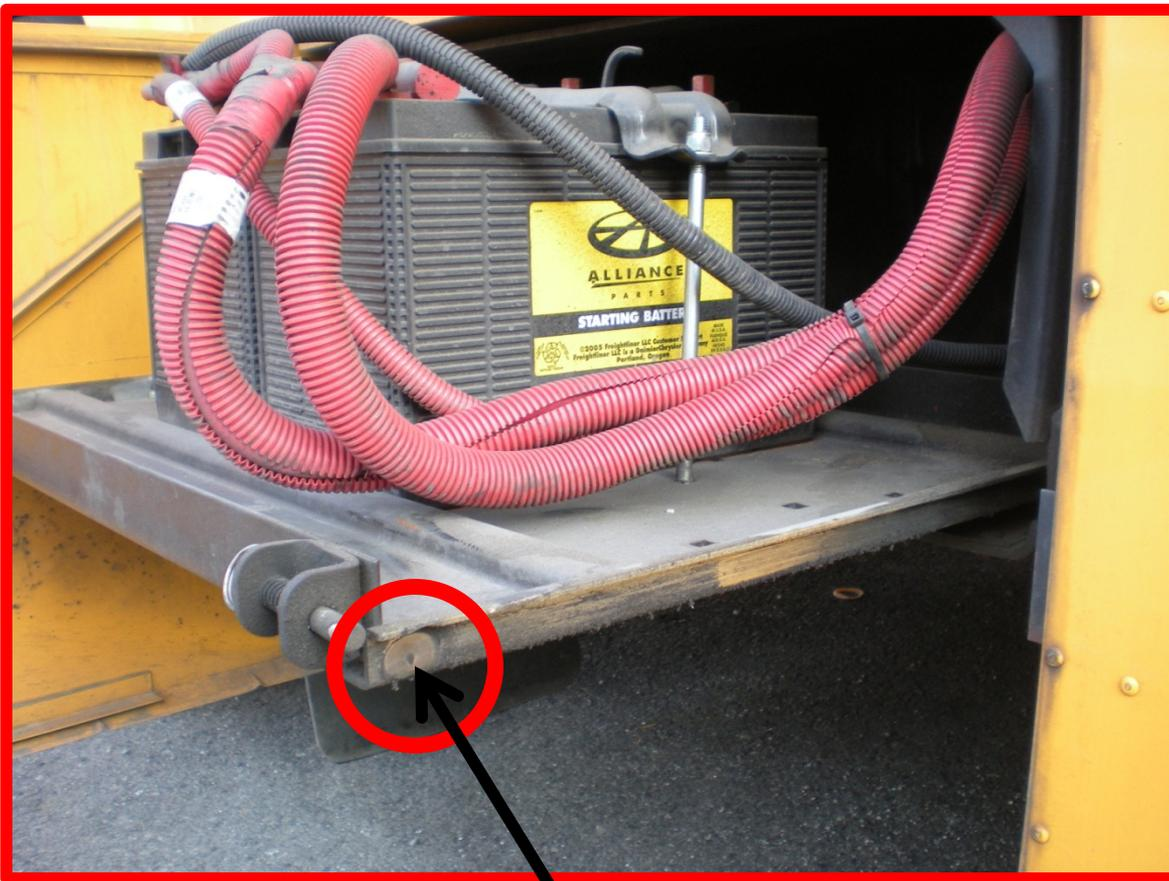
Area indicated is the where the roller rests on the battery tray slide when the box is closed. This photo shows the battery tray extended out for service.
