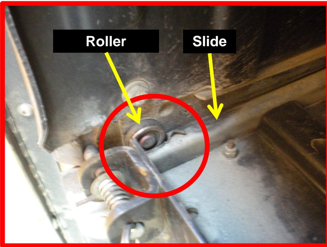
**Photo indicates tray slide roller that is wore completely through the battery tray slide. You can see roller pushed up through the slide in this photo. This photo shows the battery tray closed as if the bus was in operation.**
