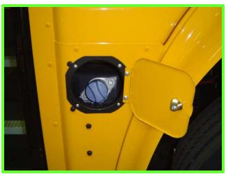
Simple – well marked compartment for DEF fluid.
