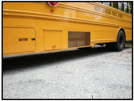
Specification Change allowing us to raise side skirts 3" more and subsequent redesign that raises side A/C condensers higher off of ground. The picture does not do justice to this but you will be impressed with this improvement.
