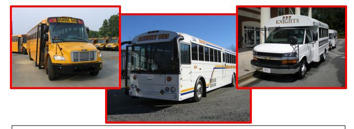
Left to Right: Saf-T-Liner C2, HDX Activity Bus, Minotour Activity Bus on GM chassis. All units have advanced design bonded curved windshields. They are nearly 4x more durable than the flat windshields in bead seal.
