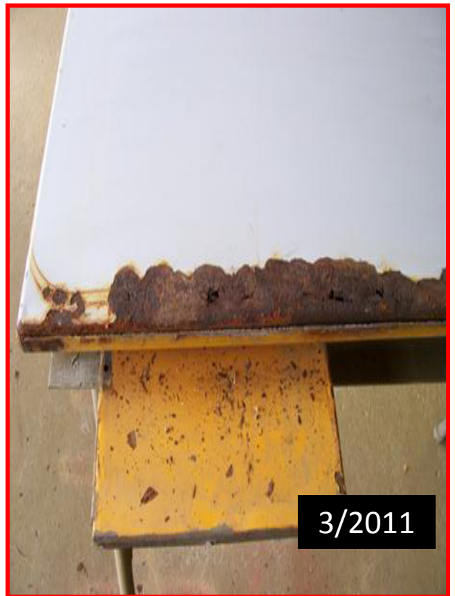
Rear interior door shown with rust perforation after salt spray tests
