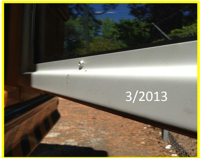
Interior door skin after salt spray tests . Bottom inside edge of door.
