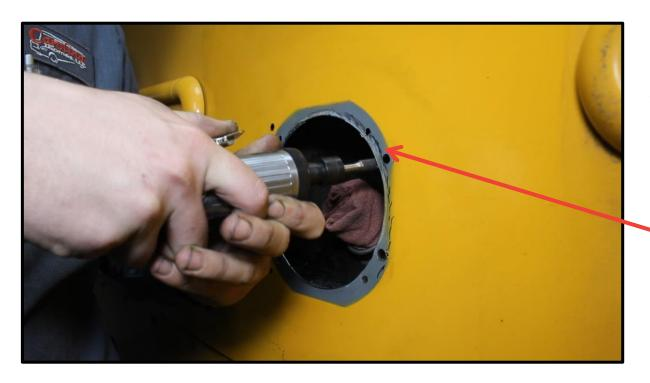
Photo depicts the body marked with a permanent marker and slight modifications being made with die grinder so the new cup will fit. **NOTE:** protective rag in fuel fill opening to prevent fuel tank contamination.
