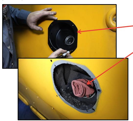
Photo depicts rag in fuel neck to prevent contamination once cap is removed. This is an important step.
