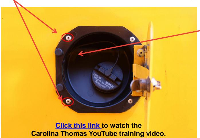
Step 16: Install fuel cap tether as shown. Remove rag from opening and install fuel fill cap and verify fit and finish.
