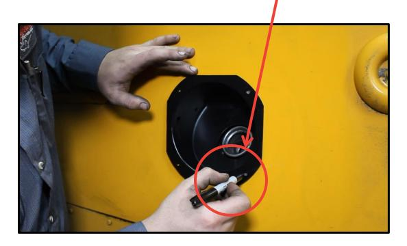
Photo shows rag removed from filler neck just for clarity. You must replace when doing any drilling to prevent contamination.
