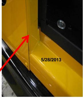
Roof Bow reinforcements are galvanized steel. Our C2 meets/exceeds "rack and static load tests for mountain usage" and rollover standards. This photo shows reinforcements in roof bows added as bus is being constructed.
