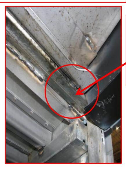
Photo shows galvanized floor tube before bus is undercoated for a better view. A stronger floor designed out most of the tubes and the rest were changed to galvanized steel.
