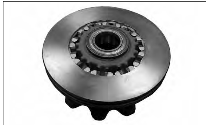
FIGURE 90 - INTERMEDIATE ELEMENTS (SPACERS) INSTALLED
