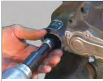
FIGURE 67 - REMOVE THE CALIPER BOLTS
