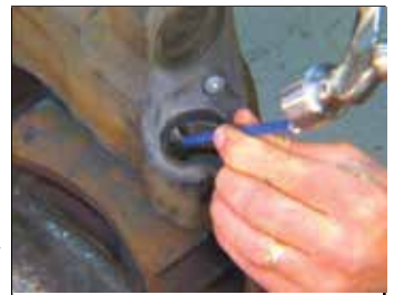
FIGURE 73 - REMOVE THE TAB THAT HOLDS THE BUSHING IN POSITION
