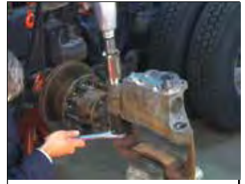
FIGURE 71 - REMOVE THE LONG GUIDE PIN
