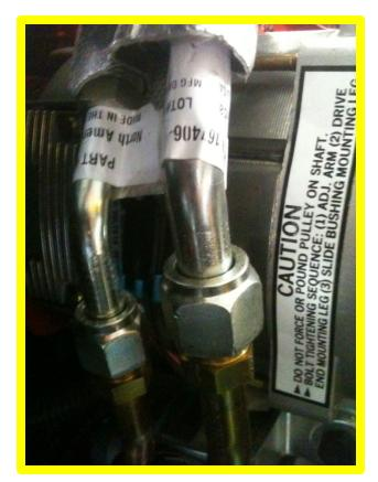
Crimped High-Pressure AC Fittings. Made in the U.S.A.
