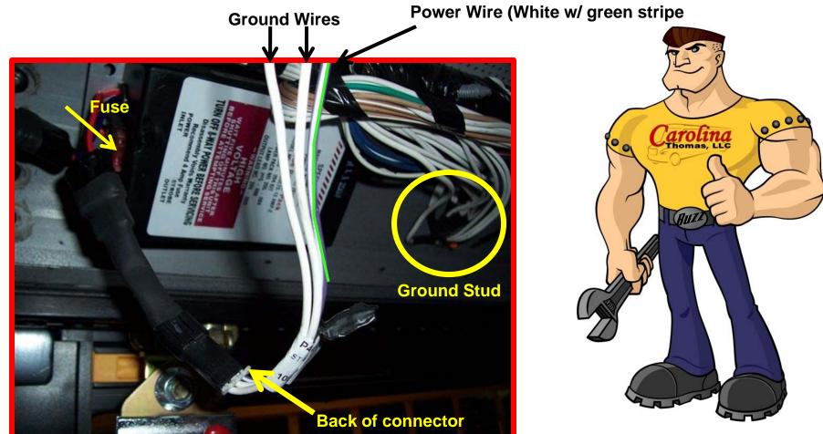
If no power at power pack your next test is at the PDM (Power Distribution Module) in driver's compartment.
