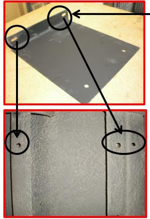
Holes shown in bus floor above storage box New storage box support bracket will bolt to existing holes in bus body floor.
