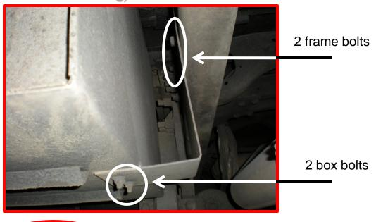
Step 3: Remove 2 bolts from original bracket and storage box floor (indicated above).
