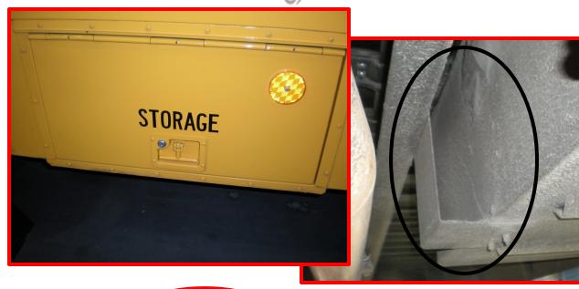
Photo on the right shows the original storage box mount and its support bracket bolted to the frame rail. Because the frame rail flexes differently than the side skirt, the storage box support bracket can crack and needs to be replaced.
