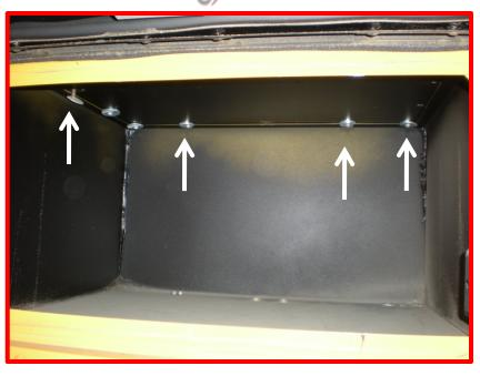
Step 9: Install top of luggage box and secure with fasteners removed previously.
