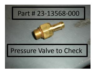
As you probably know, there is a pressure valve threaded into the surge tank. If this valve is corroded or plugged it can cause the surge tank to split. Please check this valve if you have a leaking surge tank. If the valve is plugged it needs to be replaced.
