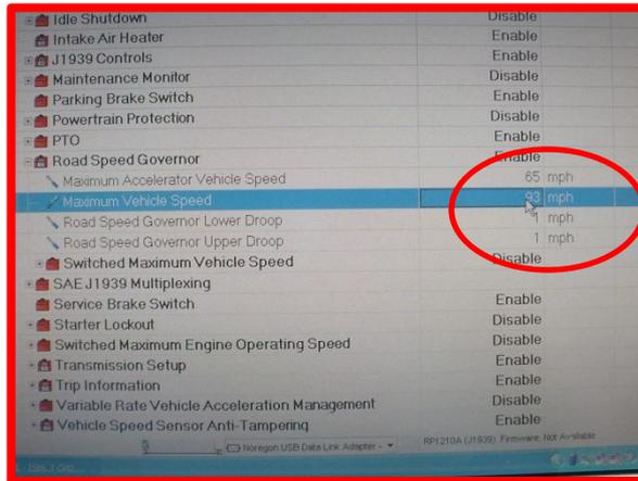
Step 8: Enter the new MPH speed required and then click on the number. **Note:** North Carolina has specific laws for buses in operation. Please adhere to these laws for any bus in-service.
