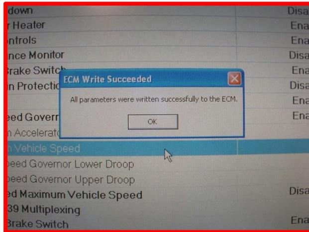
Step 14: Click Icon on left to disconnect from ECM. When this is complete it is safe to remove laptop connections with bus.
